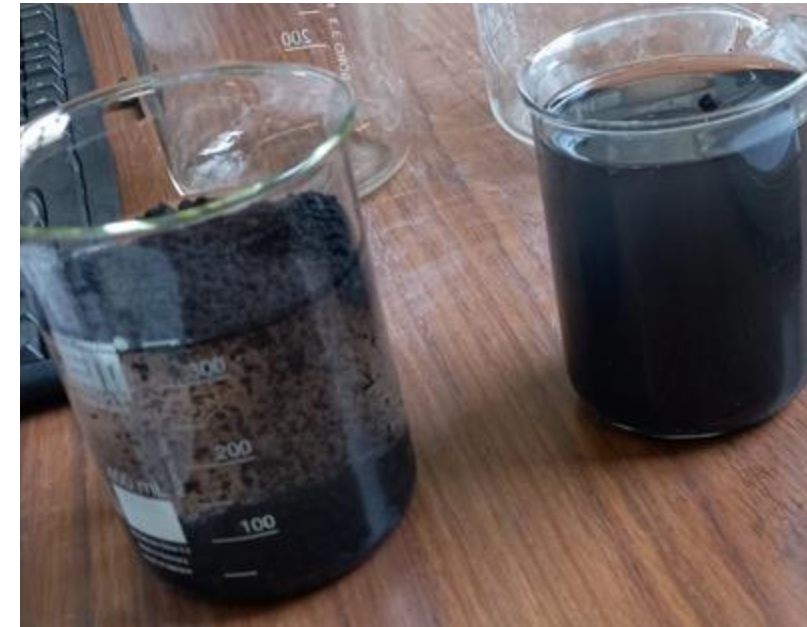
Dispersion before ultrasonication (left) and after (right).
